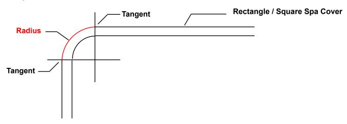
One way to measure the radius is to use a Carpenter's Square. Place the Carpenter's Square firmly against the corner of the spa cover and measure the distance from where the curve starts to the inside corner of the Carpenter's Square.
